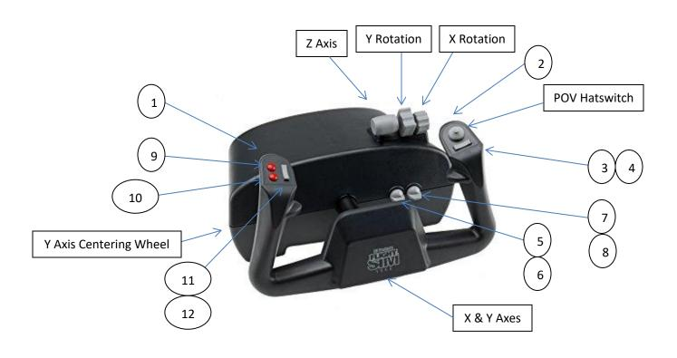
X Axis = Yoke Handle Turning Left and Right. In FS2020, assign "Ailerons Axis" to "Joystick L-Axis X"
